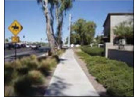
*This sidewalk on Scottsdale Road south of Doubletree Ranch Road is visually and functionally separate from vehicle paths, enhancing pedestrian safety. A landscaped buffer between the sidewalk and the curb adds shade, aesthetic appeal, and additional comfort for pedestrians.*
