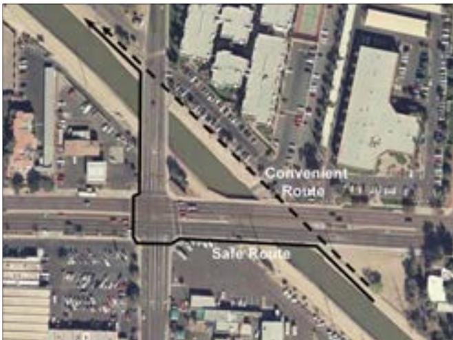
FIGURE 7-14: Safer (Solid Line) vs Convenient (Dashed Line) Crossings
