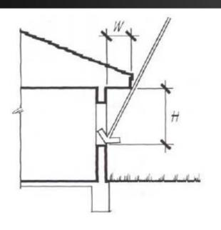
Roughly appropriate overhang dimension W can be calculated by selecting the shade line factor (SLF) from the table below and inserting in the formula:
