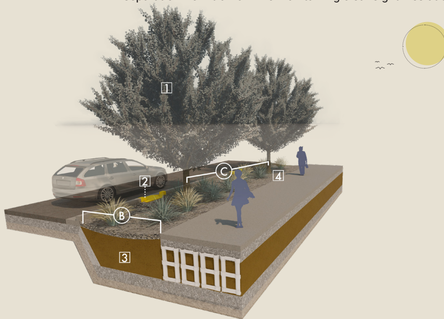
Figure 4-6. Roadway trees separated by pedestrian path
