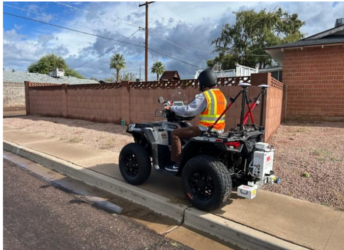
Matrix Data Collector Operating ATV Profiler
