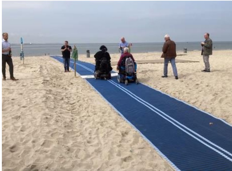
Mobi-mat, portable and removeable rollout mat for pedestrians, wheelchair users and strollers
