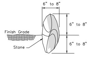
Stagger Stones To Provide A Continuous Water Bar
