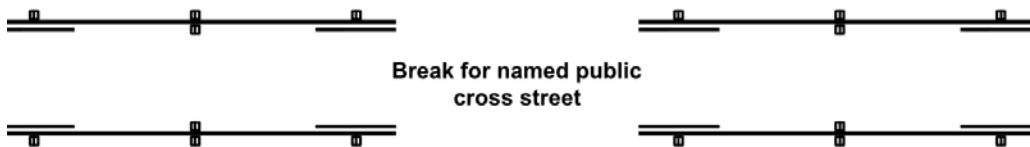
FIGURE 5-5.6 TWO-WAY LEFT TURN LANE MARKINGS
