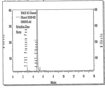
DB-ALC1 30 m x 0.53 mm, 3  $\mu m$  film thickness Column: 40°C (12 min) to 220°C at 40°C/min (5.5 min) Temp Program:
