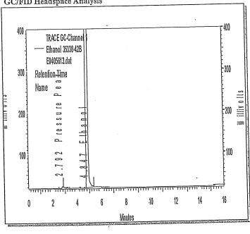
Column: Temp Program: DB-ALC1 30 m x 0.53 mm, 3  $\mu m$  film thickness  $40^{\circ}\text{C}$  (12 min) to  $220^{\circ}\text{C}$  at  $40^{\circ}\text{C/min}$  (5.5 min)
