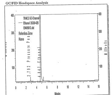
Column: Temp Program: DB-ALC1 30 m x 0.53 mm, 3  $\mu m$  film thickness 40°C (12 min) to 220°C at 40°C/min (5.5 min)
