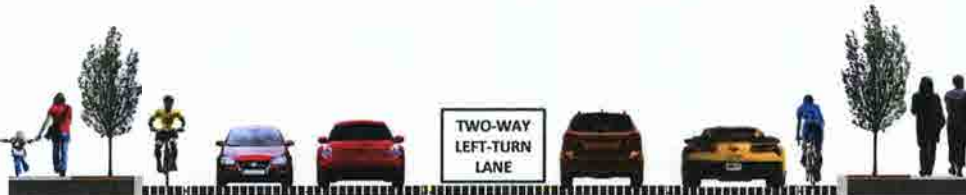
Figure 4: Generalized Street Cross-section – Major Collector
