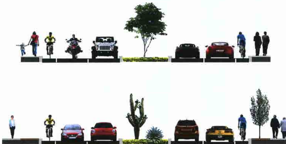
Figure 2: Generalized Street Cross-section – Minor Arterial
