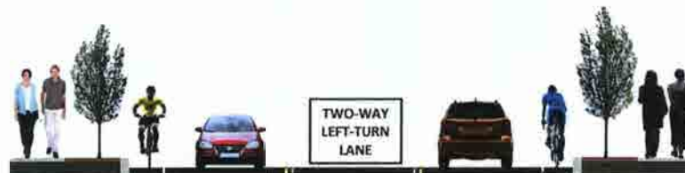
Figure 5: Generalized Street Cross-section – Minor Collector
