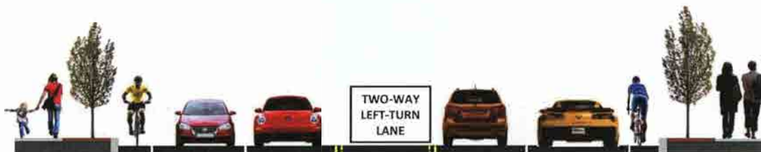
Figure 4: Generalized Street Cross-section – Major Collector
