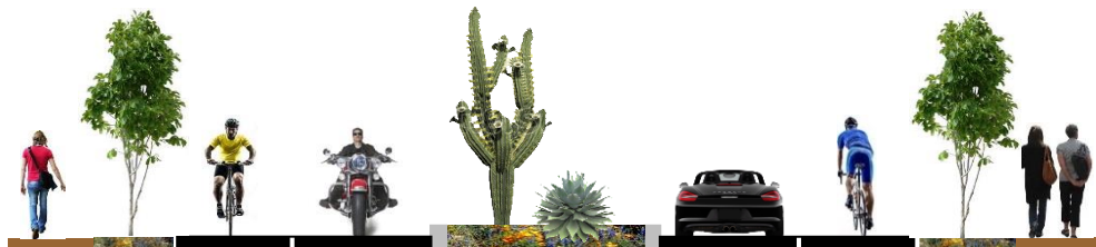
Figure 2: Generalized Street Cross-section – Minor Arterial
