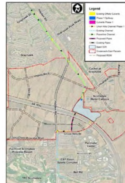
FIGURE 4.4.1 – Phase 1 Channel Concept
