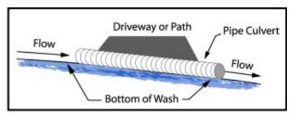
**Properly Installed Pipe Culvert**
