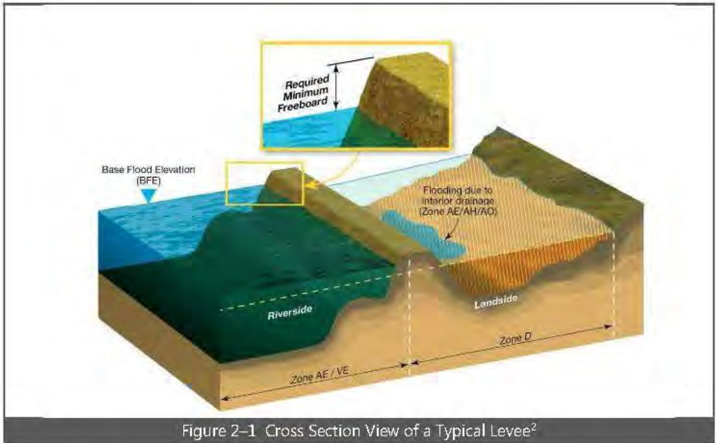
Figure 2-1 Cross Section View of a Typical Levee<sup>2</sup>
