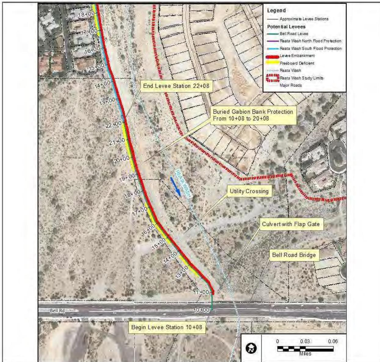
Figure 5-1 Bell Road Potential Levee Segments and Freeboard
