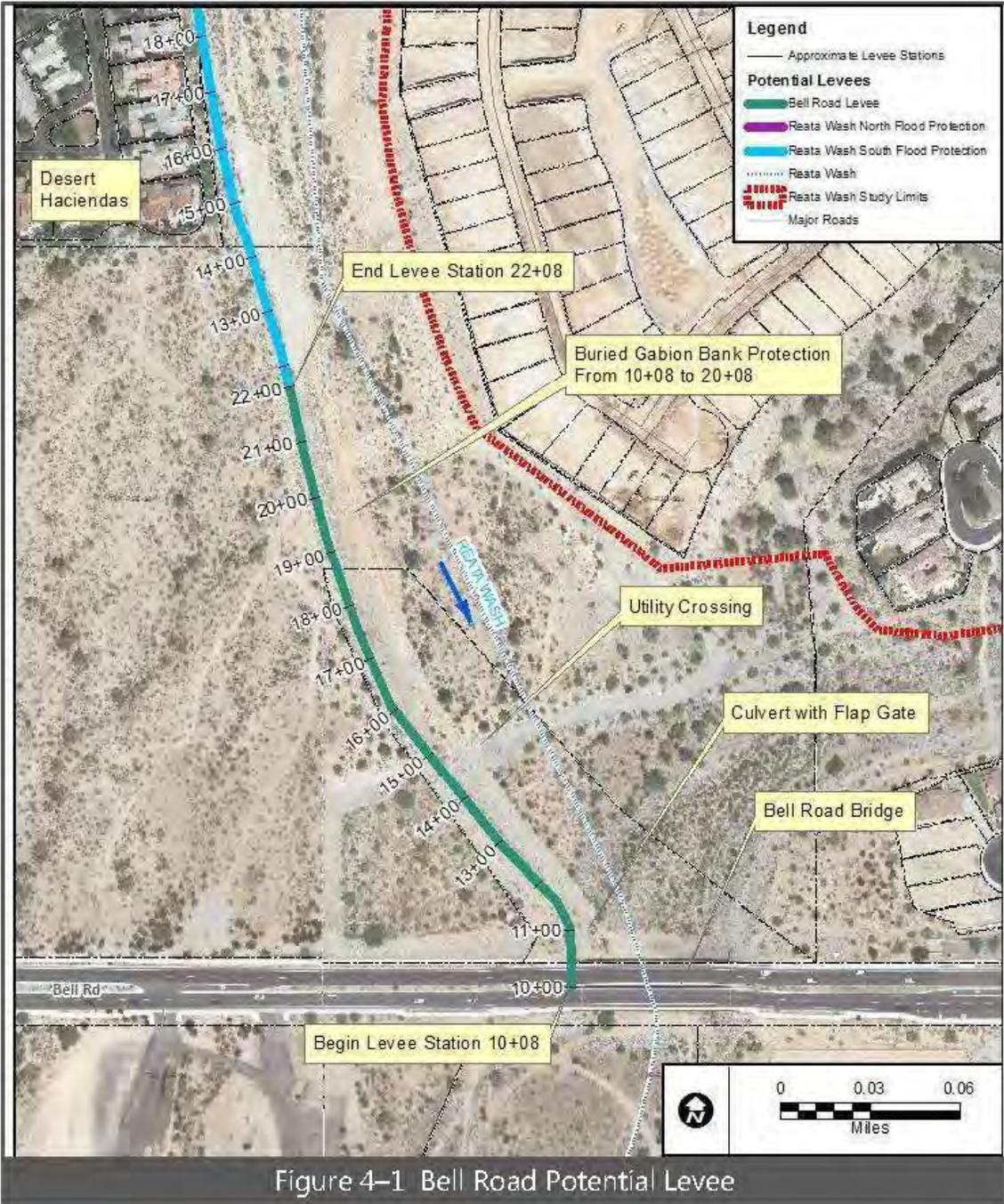
Figure 4-1 Bell Road Potential Levee
