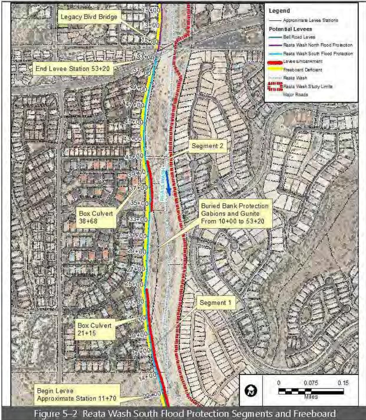
Figure 5-2 Reata Wash South Flood Protection Segments and Freeboard
