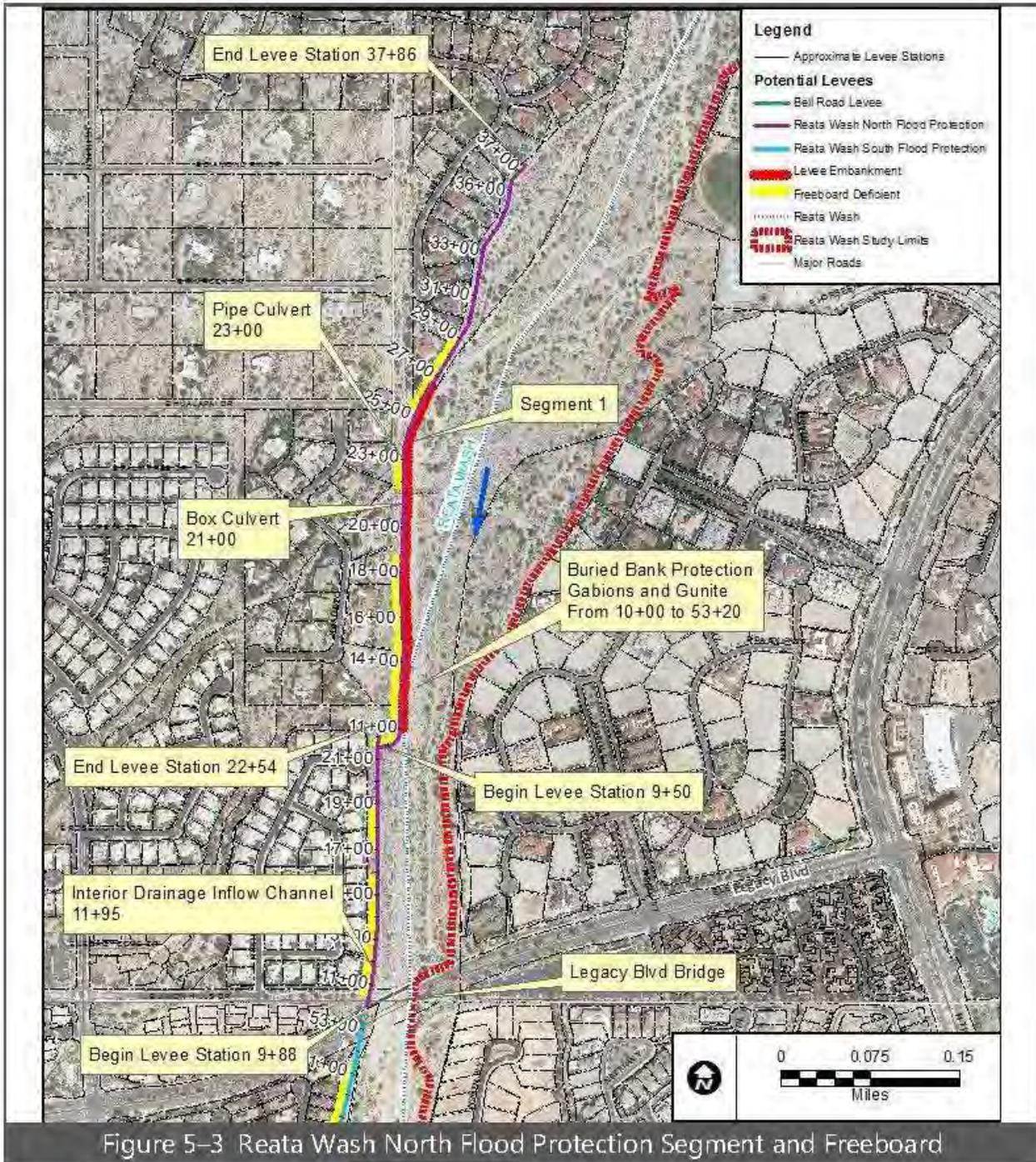
Figure 5-3 Reata Wash North Flood Protection Segment and Freeboard
