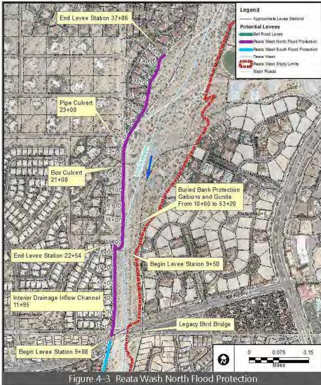
Figure 4–3 Reata Wash North Flood Protection
