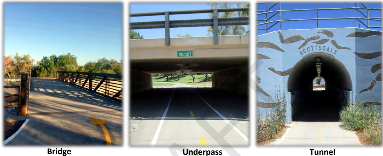
Figure P-6 Grade Separated Crossings
