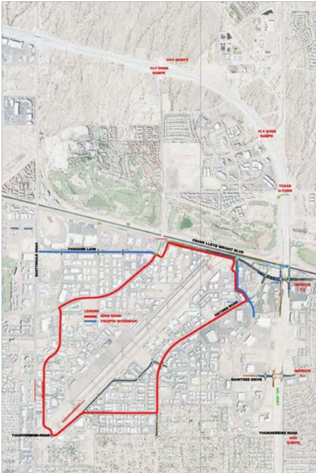
FIGURE 9-4: Airpark Area Roadway System Modifications
