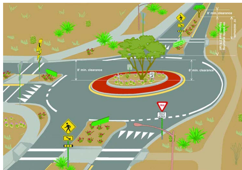
FIGURE 5.3-47 ROUNDABOUT STANDARD CONCEPT DESIGN
