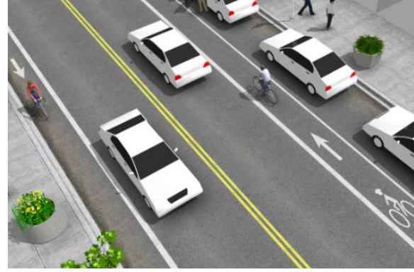
Asphalt Striped Bike Lane with on side on-street parking
