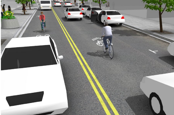
Asphalt Sharrow with one side on-street parking
