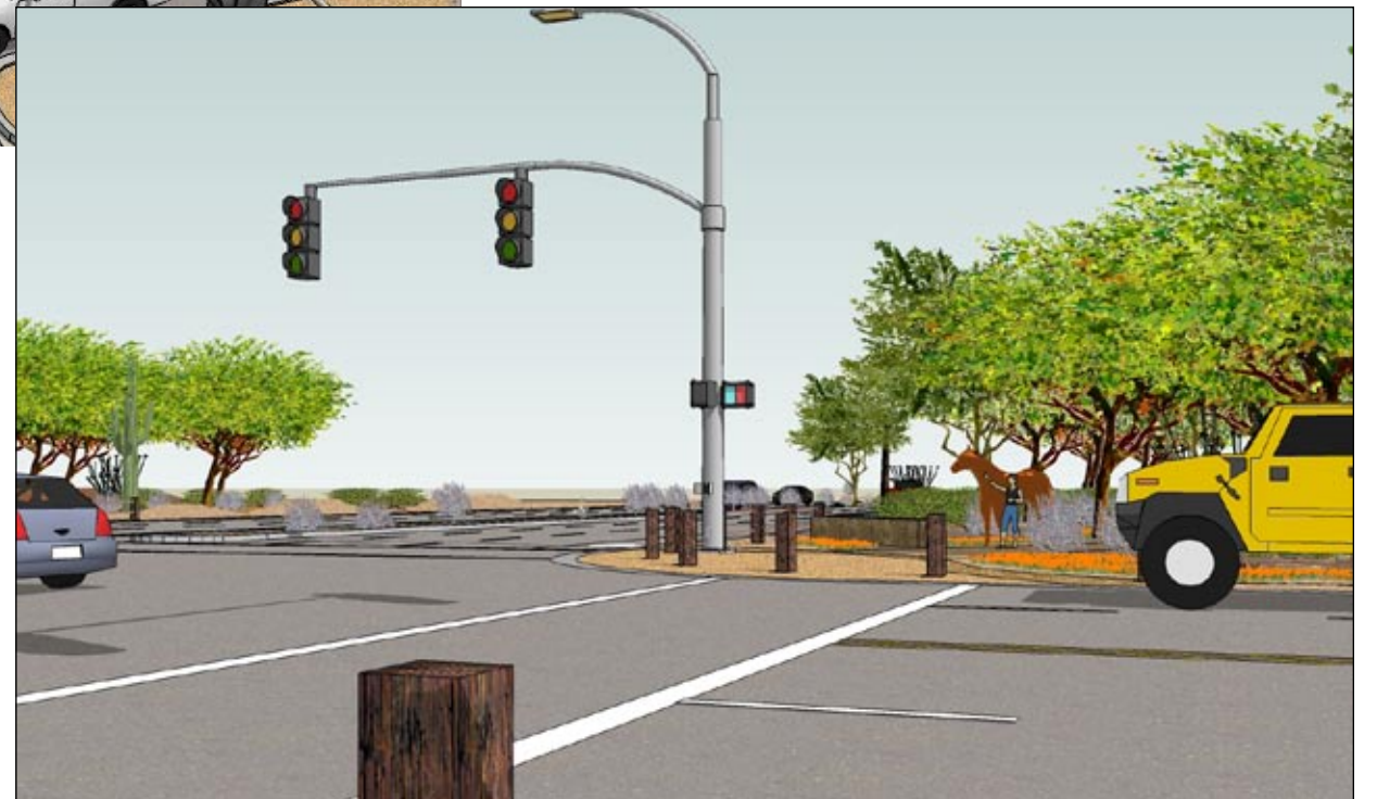
Bollards should be designed to coordinate with the metal cut-out pattern for the segment
