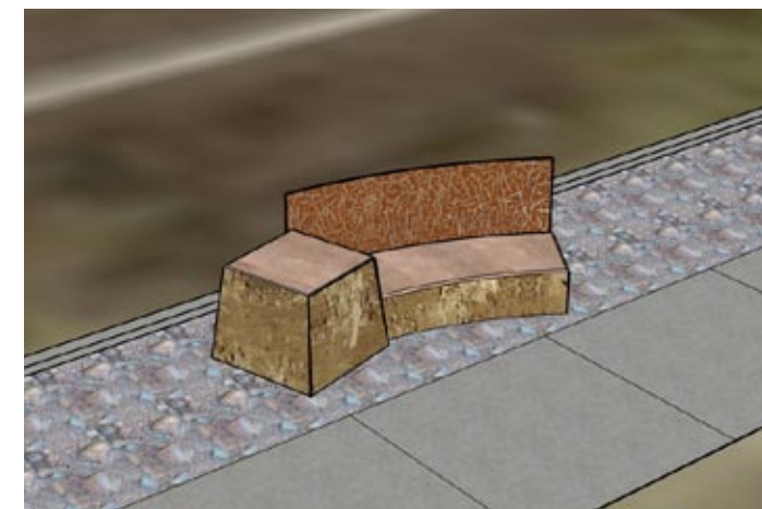
Serpentine backed bench with rammed earth finish and sculptural art plinth
