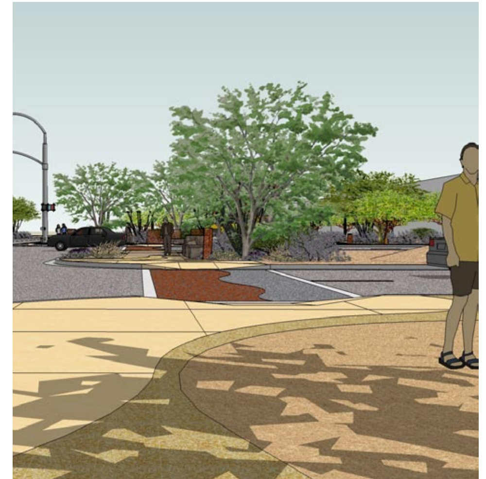
Equestrian crosswalk in Segment 5. Half of the crossing area is texturized with the other half utilizing a smooth Desert Bloom pattern
