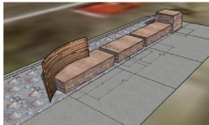
Curved backed bench with dry laid sandstone seating walls and sculptural art plinth
