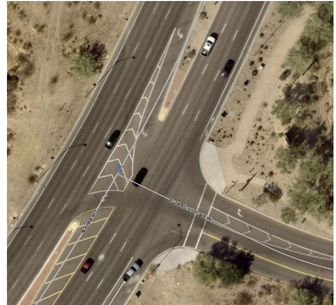
Aerial view of Pima Rd & Trailside View Dr: LILO Site (painted median)
