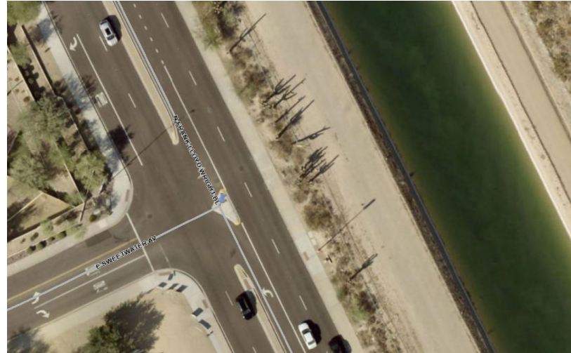
Aerial view of Frank Lloyd Wright & Sweetwater: LILO Site (raised median)
